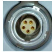
Figure 1.2.2 5pin LEMO interface
