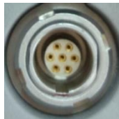
Figure 1.2.3 7pin LEMO interface
